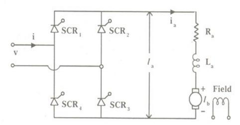
The rated motor armature current is 35 A and the armature resistance is 0.15  $\Omega$ . The a.c. supply voltage is 480 V. The motor back emf constant is  $k_b \phi = 0.45 \text{ V/}$
